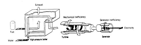
B Conventional process-steam system requires the equivalent of 2½ barrels of oil to produce 8,500 lbs of process steam.
