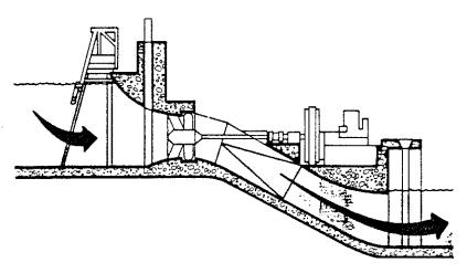
The tubular-type turbine uses a conventional horizontal propeller turbine and an attached generator located outside the water passage.
