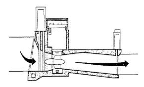
The energy efficiencies of turbines run generally between 75 and 95 percent. Francis turbines have very high efficiencies of up to 95 percent when operating at designed pressures, but they are generally more expensive than other types and quickly become inefficient as pressure and flows vary from design specifications. Impulse turbines have flatter efficiency curves and generally are less expensive.
