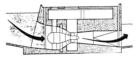
The bulb-type turbine generator is in a bulb-shaped watertight steel housing located in the center of an enlarged water passage.
